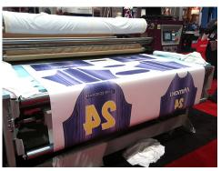
Sublimation is a unique technology in which colors, designs, and logos are heat-infused directly into fabric. Sublimation results in an image that will not crack, peel or fade when washed. Therefore, sublimation is ideal for products such as team apparel, which undergoes a lot of physical stress and numerous washings in its lifetime.
